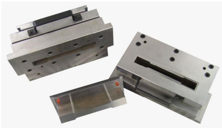
Dismantled punch tool for sheet metal tensile specimens (on tool parking desk)
